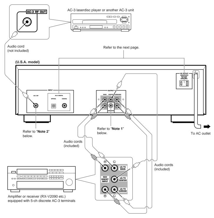
Note 1) If this unit is connected to the RX-V2090, no connection is needed to this terminal. By the output mode selections on function C2 to C5, low frequency signals including signals from the LFE channel can be output from the main L and R speakers. (See page 10 for details.)
