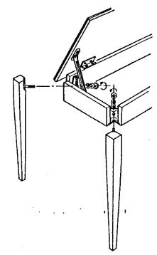
\*The nuts shown secure the legs to the bench base. Please check all four legs, Tighten the nuts indicated if a leg seems loose.
