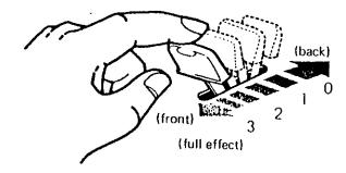
There are tone levers to control various sounds of the keyboards and pedals. They are divided into three groups, the upper keyboard, the lower keyboard and pedals, so that different tones can be set for each.
