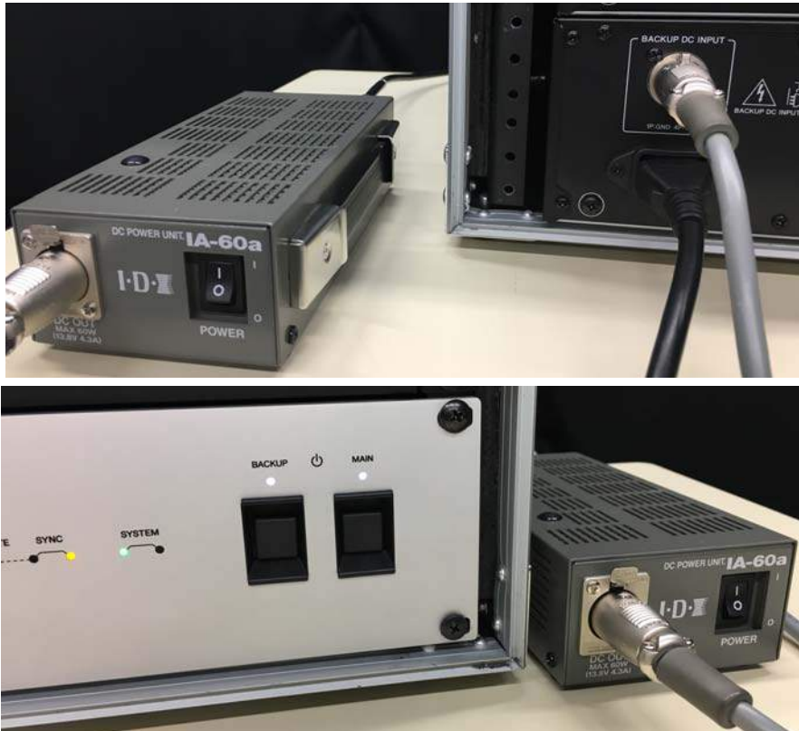
[Redundant DC Power Unit]
