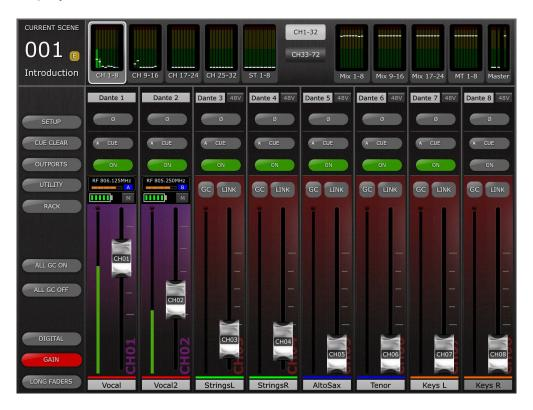
The fader will control the output gain of the wireless receiver(RX) channel. Above the fader, the current battery status of the wireless microphone is displayed. To the right-side of battery indicator, the Mute status of the receiver audio output is shown (if available on the wireless
