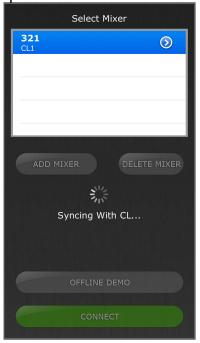
The message "Syncing With CL..." will appear while StageMix is obtaining parameters from the console. After this process is complete, the Mixer window will appear and StageMix is ready to be used.
