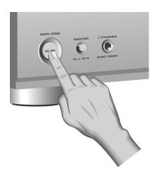
This unit is set to the standby mode and consumes a small amount of power in order to receive infrared signals from the remote control. To turn on this unit from the standby mode, press the desired **SCENE** buttons (or **SCENE**) or **MAIN ZONE ON/OFF** on the front panel (or **POWER** on the remote control). See page 25 for details.
